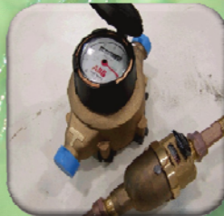
Water and irrigation meters
